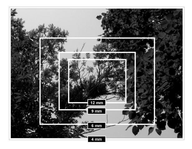
**Figure 24 - The effects of lens focal length upon field of view.** This example illustrates the differences in the field of view depending upon lens focal length. Camera capability and lens quality were factors that had to be reconciled in a manner that best met the study objectives. This image of eight week old Great Blue Heron chicks was taken from a distance of ~ 6.5m. The nest is approximately 1m wide. (Photo: Andy Von Duyke)
