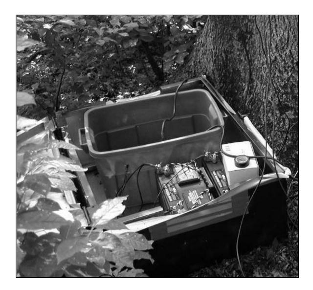
**Figure 9 - Weather and theft protection.** A welded steel security box, chained to the base of each study tree, protected recording equipment from theft, vandalism, and the elements. The open lid is visible on the left side of the box and was sealed using weather stripping and duct-tape. The purple plastic tote provided additional weather protection. (Photo: Steve Kittelson, MN-DNR)
